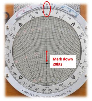
Next rotate the disc to place the mark directly down from the centre. Read the wind direction under the index and speed down from the grommet.
