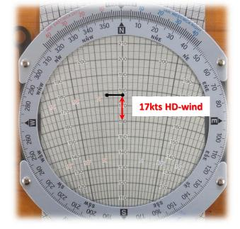
Next, rotate the disc to place RWY HDG under the index. Draw a straight line from the mark to the centreline. Read the head-wind component between the line and the grommet (17kts).
