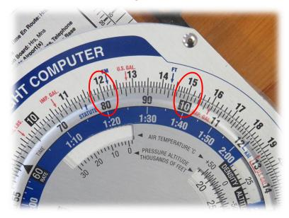
First step, rotate '10' on the inner scale till it's under '15' on the outer scale. Find '8' on the inner scale and above that, read the altitude gained after the climb (12Øft).
