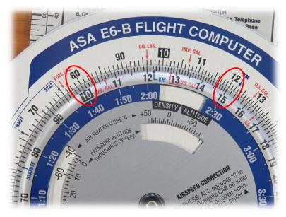
First step, rotate '15' on the inner scale till it's under '12' on the outer scale. Find '10' on the inner scale and above that, read the time in minutes on the outer scale (8 minutes).
